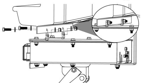
5. Lower the front end of the step down to expose the marked holes. Take a drill motor (a right-angled drill motor will make this easier) with an 11/32" drill bit and drill out the marked holes. Remove all burrs. Lift the step back into position. Take the remaining 5/16" hardware and securely tighten the Front Steel Brackets to the vehicle.
