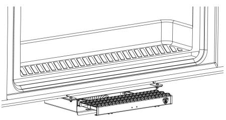
7. Now your step is ready to go. Push the step in to lock in its closed position. Push it again to deploy it. We recommend using a garage door opener silicone spray on the rails from time to time to insure smooth operation of the step.
