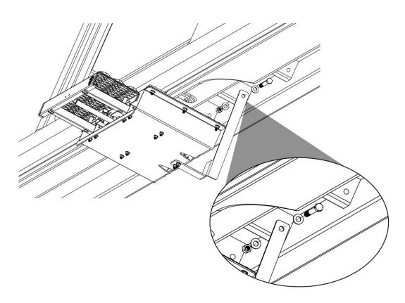
3. Take the entire step assembly and lift it up inside the vehicle behind the side door. It is highly recommended to use a floor jack or something to rest the step assembly on while completing this step. Make sure the Rear Steel Bracket is up against the middle cross member as shown. Take the 1/2" hardware and assemble it to the vehicle but only hand tighten. This 1/2" bolt assembly will be tightened in step 7.
