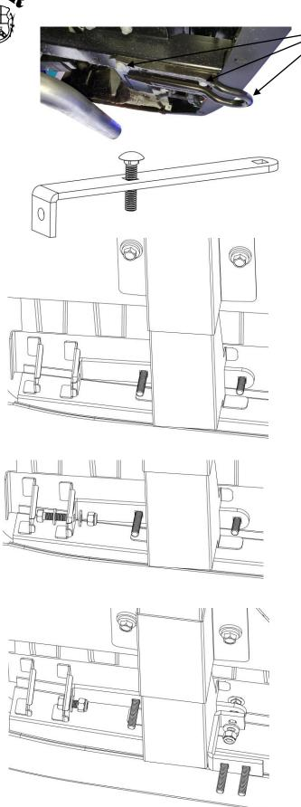
Newer models have this Tow Hook bracket that needs to be removed before the step can be installed. Remove the 2 bolts and the factory Tow Hook bracket and proceed to step 2. CARA
