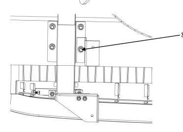
6. A very important step in the installation process, make sure to tighten this nylon lock nut so the bolt only comes through an 1/8". If this nylon lock nut gets over-tightened, it will be very difficult to install the front bolts later in step 10.
