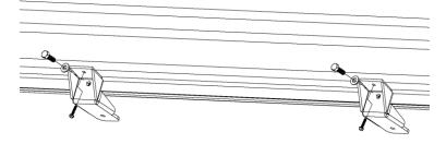
7. Place the step assembly back into place. Use the 5/16" X 1" hardware used in step 1 to reinstall the step assembly. Securely tighten the hardware. If the holes do not line up, loosen the other hardware enough to get all hardware aligned and than securely tighten the hardware.
