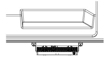
2. From underneath vehicle, position the step assembly centered on the open step area of the van as shown. You will need to use a floor jack or some way to hold the step in this position for the next step.
