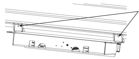
4. With the step assembly in position and the Front Mounting Brackets up against the body metal, mark two holes using the holes in the Front Mounting Brackets as a guide. Lower the step assembly and drill out the marked holes with an 11/32" drill bit.
