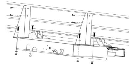
6. Place the Front Mounting Brackets back into place. With the Blind Retainer Nuts installed, use the 5/16" X 1" bolts with the flat washers and tighten both brackets to the vehicle. Take the two  $\frac{1}{4}$ " self-tapping screws and install them through the  $\frac{1}{4}$ " holes on the top of the Front Mounting Brackets. An impact wrench will make this easier.
