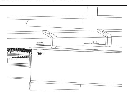
6. Take the two 1" long 5/16" bolts with washers and nylon lock nuts and securely tighten the "C" shaped steel brackets to the vehicle's rocker panel.
