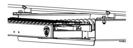
7. Remove the bolt assemblies that hold the "C" shaped steel brackets to the pan. Take the cover plate and slide it between the pan and the "C" shaped steel brackets. Align the holes and reinstall the bolt assemblies just removed. Take the remaining 5/16" X ¾" bolts with washers and nylon lock nuts and securely tighten the cover plate to the pan.
