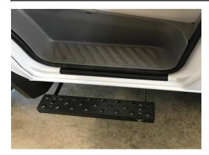
6. Re-install your step and with the 3/16" Allen wrench and ½" socket fully tighten all four button head screws.
