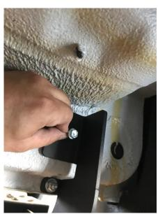
7. Fully tighten both 5/16" hex bolts to pinch weld. Finally with a 3/8" socket install the #14 self-tapping screws to both brackets and be careful not to over tighten them. Your step is now fully installed follow the same procedure for other side.
