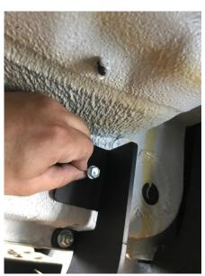
7. Fully tighten both 5/16" hex bolts to pinch weld. Finally, with a 3/8" socket install the #14 self-tapping screws to both brackets and be careful not to over tighten them. Your step is now fully installed.
