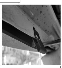
4. With both holes drilled out use a flat head screwdriver to pry on plastic trim and slide in the U-nuts.
