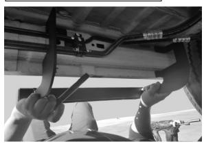
2. With step assembled, place step in the desired location avoiding any A/C lines as shown (Passenger vans only) Avoid any bumps or indents to allow both brackets to be parallel to each other. With a marker mark both holes for the 5/16" mounting hardware; top holes do not need to be marked.
