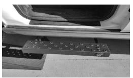
6. Re-install your step and with the 3/16" Allen wrench and ½" socket fully tighten all four button head screws.
