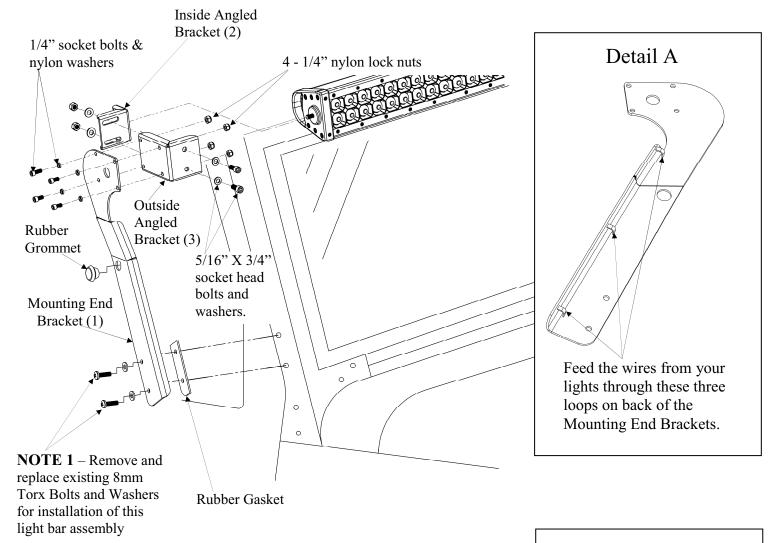
**TOOLS AND MATERIALS NEEDED:** Wrench for T40 Torx and 3/16" Allen wrench, Loctite, 5/32" Allen wrench, 7/16" wrench/socket, ½" wrench/socket.
